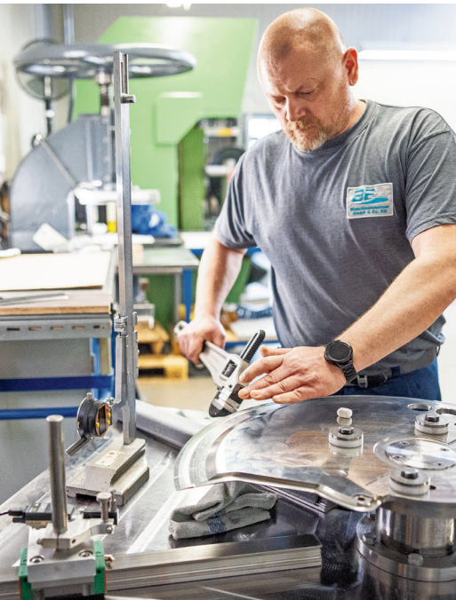
David Nickel straightening a machine knife, using the dial indicator to check that the tolerance of 0.2 millimeters is maintained.
